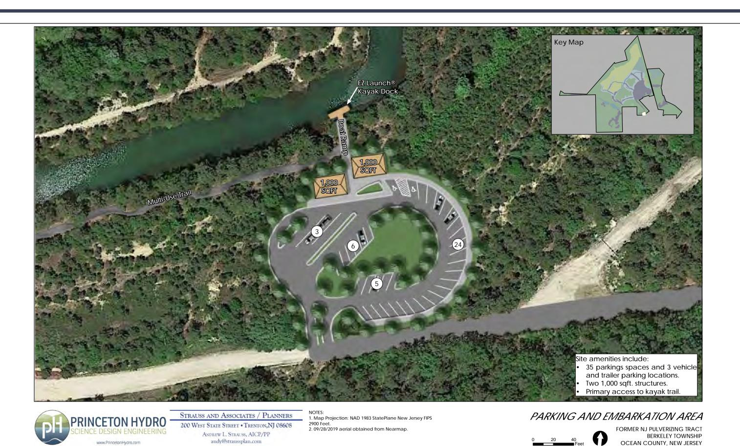
FIGURE 10: Located off Hickory Lane the proposed parking and embarkation area will provide public access to land and water trails, and incorporates 35 spaces with additional trailer parking, picnic pavilions, restrooms and a kayak-canoe launch. Additional parking and trailhead areas will be developed in several phases.
